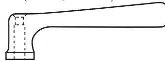
Height _____ (max) 40mm Centre hole in top face (when supplied), 6mm x 10mm c/s.
